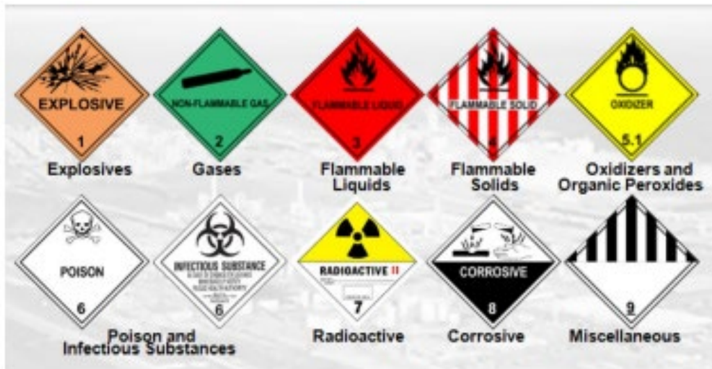
Figure 3: Hazardous Materials Classification Placards
